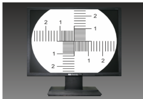
Image section with eyepiece f=14,7\text{ mm}
