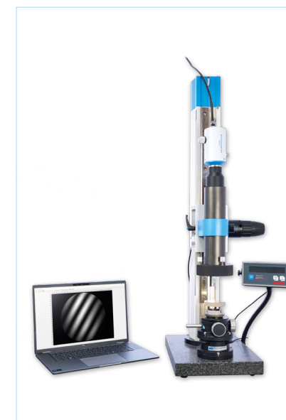
MEASURING STATION FOR RADIUS DETERMINATION AND TESTING OF PLANE AND SPHERICAL SURFACES IN INCIDENT LIGHT
